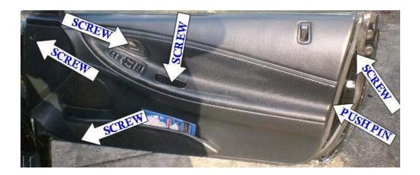
Then carefully pull away the clips along the bottom edge of the door-card and lift and remove. Next, reach down behind and unplug the two multiplugs from the door switch and electric mirror controls. Then by twisting the door card, you are able to coax the door handle through the hole without any need to disconnect it from the metal rod.
